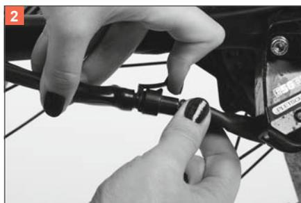
6. Check on the display at the control element that the system has been switched off (1). Only then should you connect the motor to the cable loom. Do this by connecting the motor plug to its counterpart in the cable loom (2). Ensure that the connection at the plug is not reversed (geometric alignment). Always connect the plugs slowly and with care, without using force.
